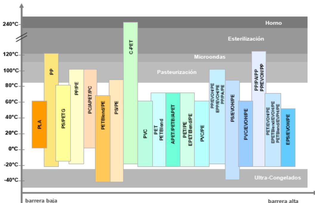
Figure 2: Range of multilayer structure applications
