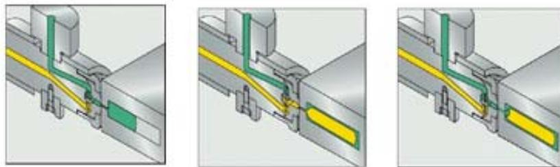
Figure 4: Co-injection process steps.
